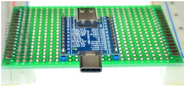
Figure 5: Solid Mounting on prototype PCB
